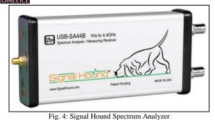
The Signal Hound Tracking Generator has 19 selectable step sizes from 10 Hz to 10 MHz and 16 step sizes from 100 Hz to 10 MHz above 4 GHz. The amplitude ranges from -30 to -12 dBm. (-30 to -10 dBm typical) with a step size of 1 dB.
