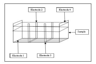
Fig.2: Schematic of the measurement cell
