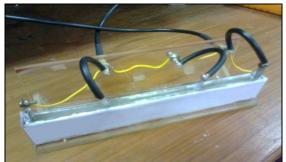
Fig. 1: Four probe impedance measurement cell
