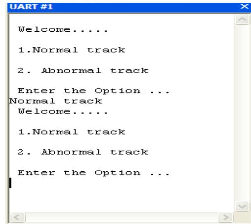
MODE 1 is selected, UART displays to select the desired track 1 or 2(for displaying normal or abnormal track).then the UART display when normal track activated no indication is occur.
