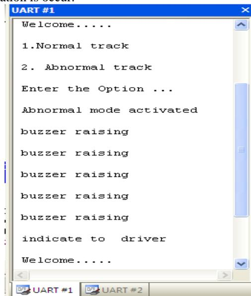
MODE 2 is selected ,UART displays to select the desired track1 or 2(for displaying normal or abnormal track ).then the UART display when abnormal mode is activated buzzer become raising and indicate to the driver.
