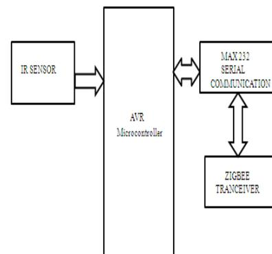
Fig-3. Block diagram of sensor node
