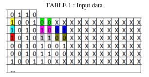
A 274 bits register is needed to memorize the March test data. Table 1 gives for example the data-base implantation of the March test C-.
