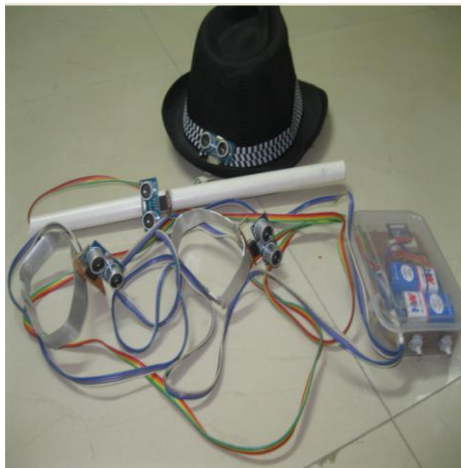
Fig.9 Complete Assembly of the Microcontroller based Virtual Eye for the Blind
