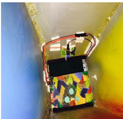
Fig.4. Open close plate with three inductive proximity sensors for metal waste detection
