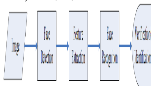
Fig. 1: Configuration of a general face recognition structure
