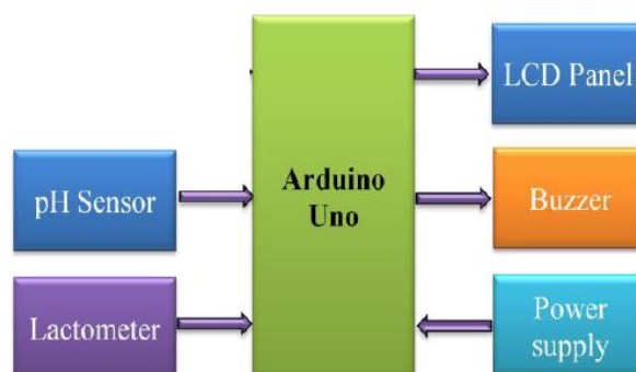
Figure2: Block diagram of Milk parameter measurement system
