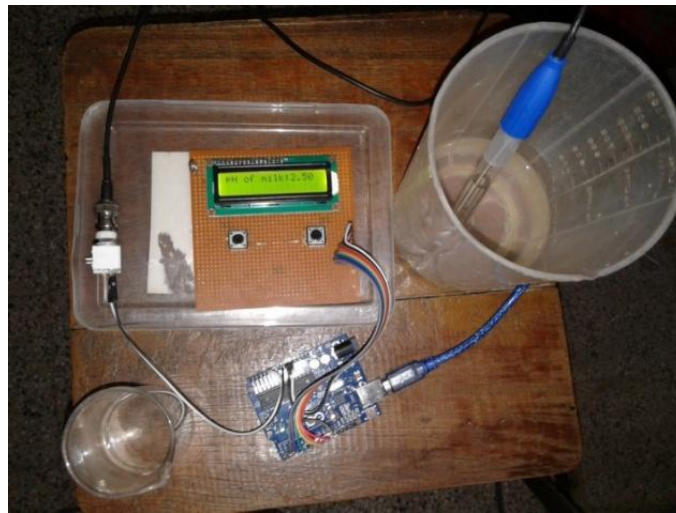
Fig.4: The pH measurement setup
