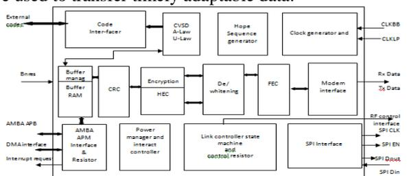
Figure 3: Bluetooth baseband core diagram
