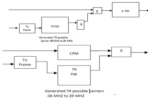
Figure 5: Frequency hopping transmitter and receiver.
