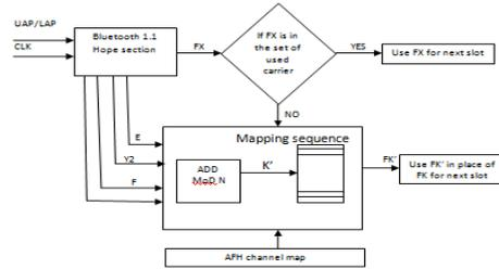
Figure 4: Block diagram of adaptive hop selection mechanism.
