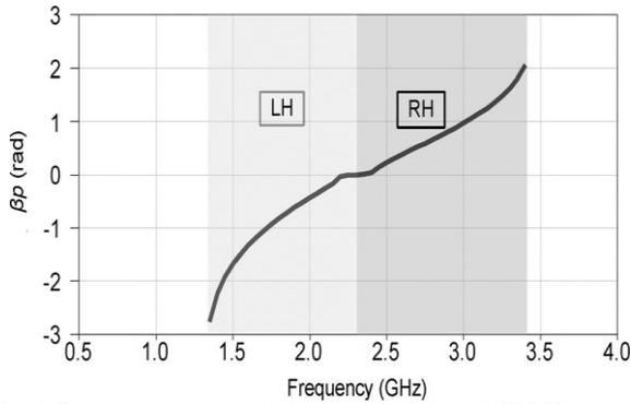
Fig. 3. Dispersion relation calculated for the balanced CRLH unit cell with dimensions
