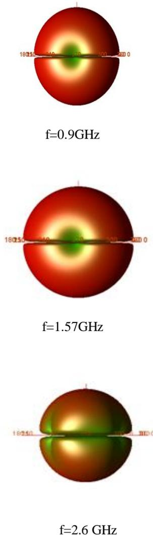
Fig.6.Simulated normalized radiation pattern for loop antenna
