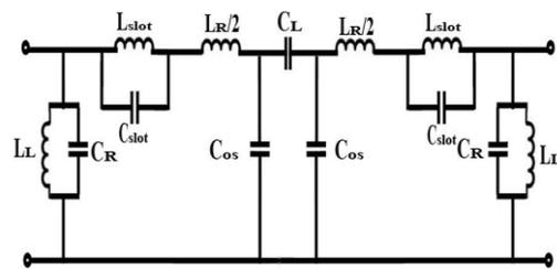
Fig 1. A Equivalent circuit of CRLH transmission-line unit cell
