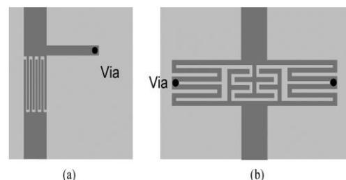
Fig. 2. (a) CRLH unit cell presented (b) Modified CRLH unit
