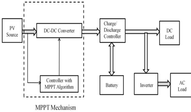
Fig. 1. Block diagram of Battery charging system
