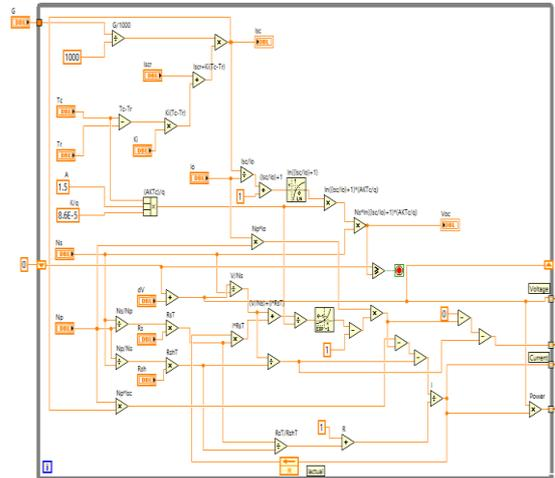
Fig. 5. PV panel simulation
