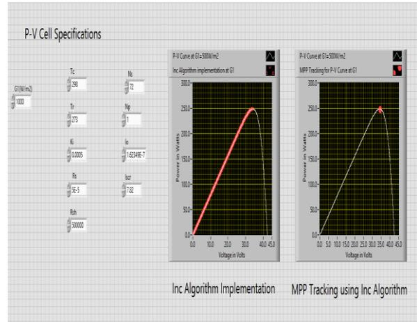
Fig. 7. PV characteristics of InC algorithm
