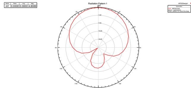
Fig. 9. E - Plane plot for Circular Patch Antenna with 0<sup>0</sup> phase shift
