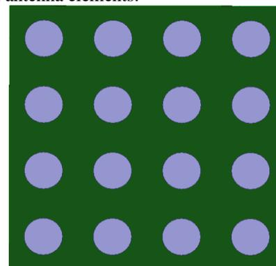
Fig. 3. 4x4 Circular patch array
