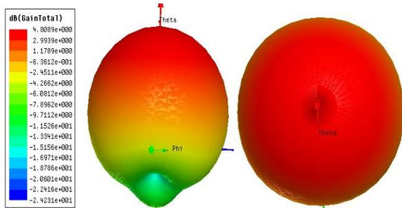
Fig. 13. 3D-Polar Plot for circular patch antenna
