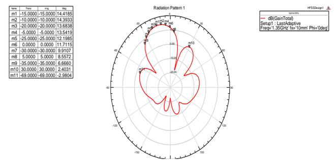
Fig. 11. E - Plane plot for Circular Patch Antenna Array with 10<sup>0</sup> phase shift for individual element
