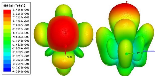
Fig. 15. 3D-Polar Plot for circular patch array at 10° phase shift for individual element
