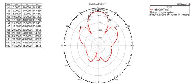
Fig. 10. E - Plane plot for Circular Patch Antenna Array with 0<sup>0</sup> phase shift for individual element
