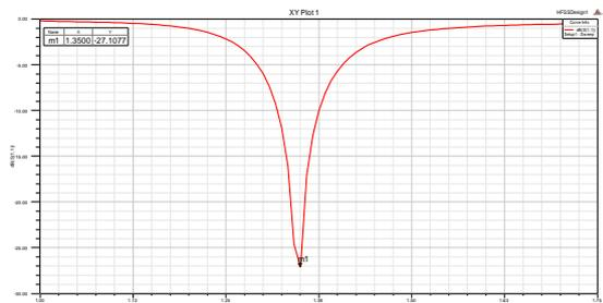
Fig. 6. Return Loss plot for Circular Patch Antenna Array
