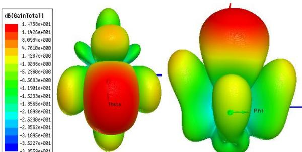
Fig. 16. 3D-Polar Plot for circular patch array at -10° phase shift for individual element
