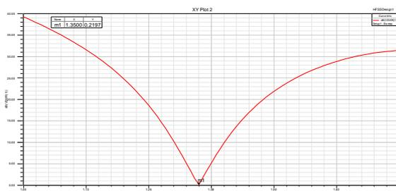
Fig. 7. VSWR plot for Circular Patch Antenna
