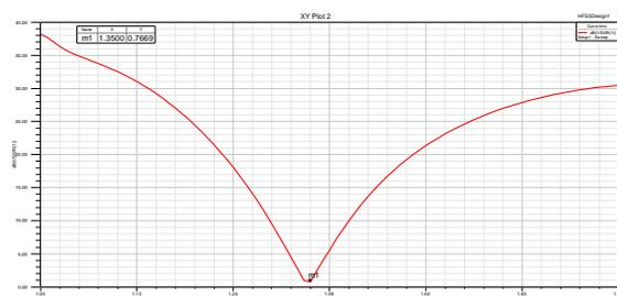
Fig. 8. VSWR plot for Circular Patch Antenna Array
