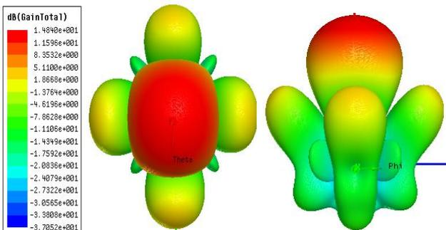
Fig. 14. 3D-Polar Plot for circular patch array with 0° phase shift for individual element
