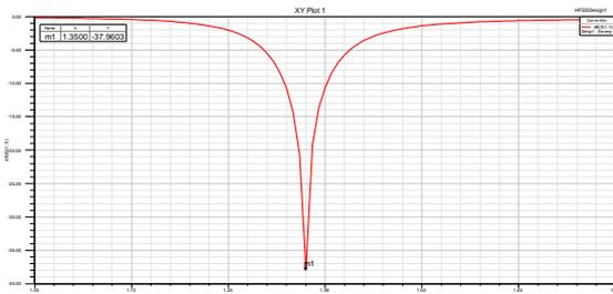
Fig. 5. Return Loss plot for Circular Patch Antenna
