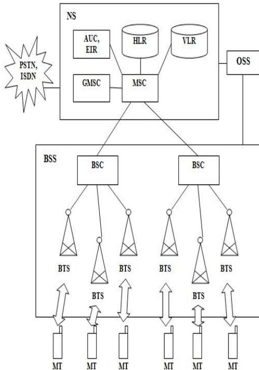
Fig1. GSM Block Diagram
