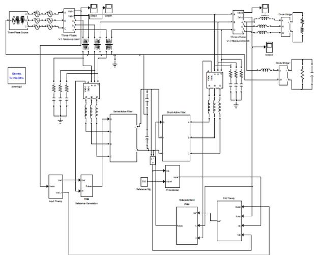
**Fig. 3 Simulation Circuit of UPQC**
