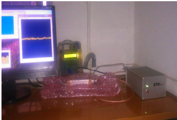
Fig. 9. Data acquisition system with control circuit and CALLISTO
