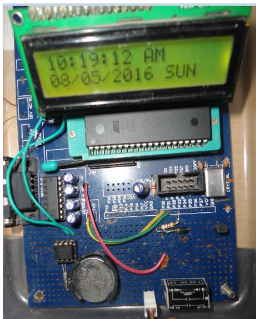
Fig10. LCD display connected to RTC shows time, date and day.
