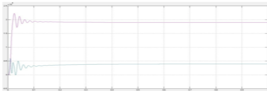
Fig.9. Active And Reactive Power with PFC
