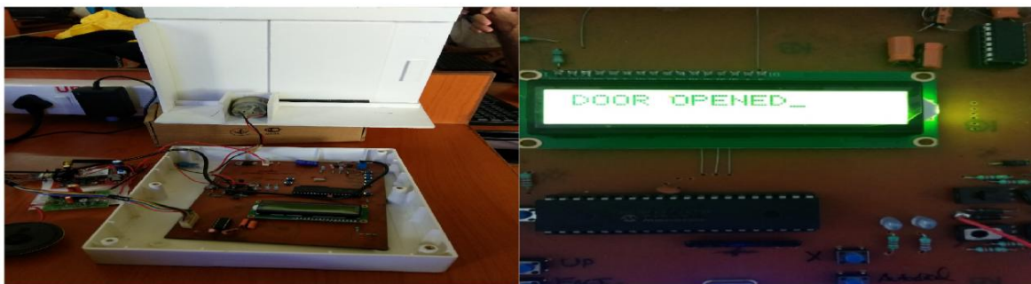
Figure9. Door accessing via SMS.
