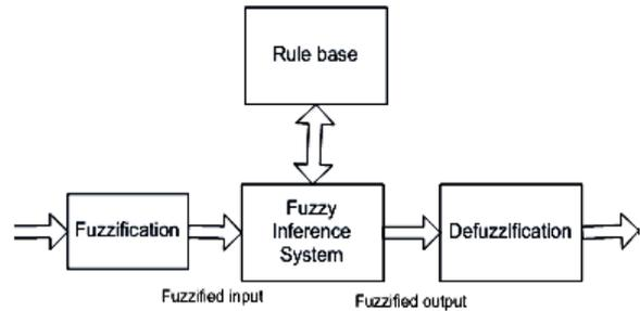
Fig.2 Block diagram of a fuzzy control system
