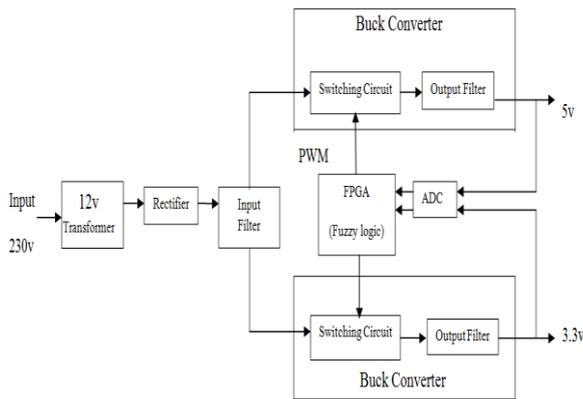
Fig.1 Block diagram of digital controlled SMPS
