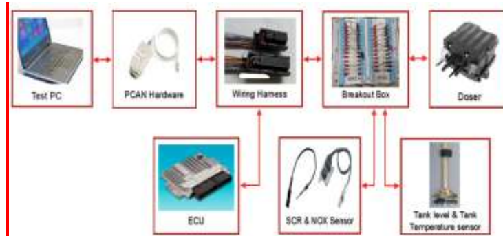
Figure-2 Block diagram of Manual test bench setup for UA2 Doser
