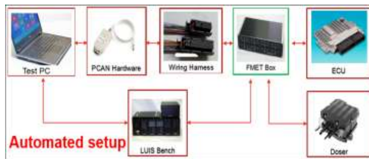
Figure-3 Block diagram of the HIL system
