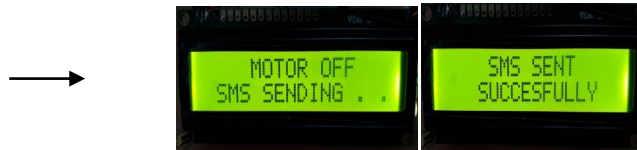
Fig 10: Motor OFF, The SMS is sent successfully to registered phone number.
