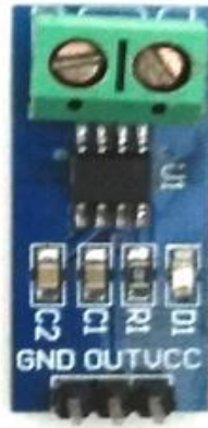
Fig 5: ACS712 Current sensor
